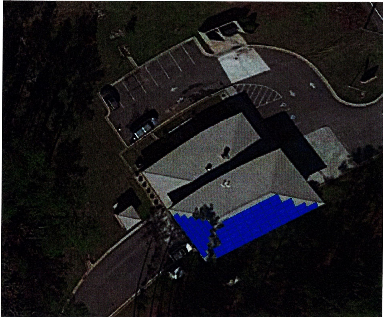
Figure 1: Solar roof-mounted system on south/southwest roof surfaces
