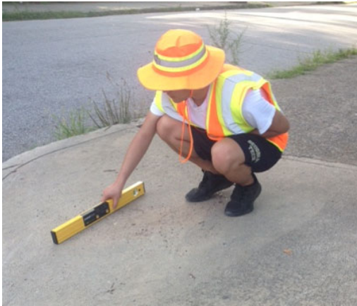
Figure 5. Researcher Measuring Curb Ramp Running Slope with Level, Left Example Minimum Measurements for Curb Ramps, Right (AASHTO, 2004)
